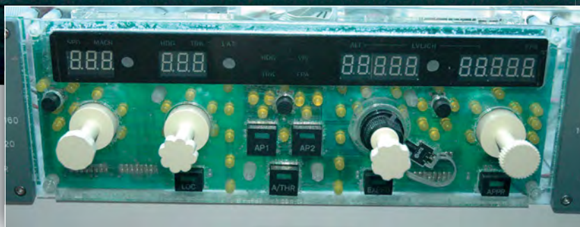
The FCU with its front panel removed. Note the altimeter 100/1000 switch placed on the right
