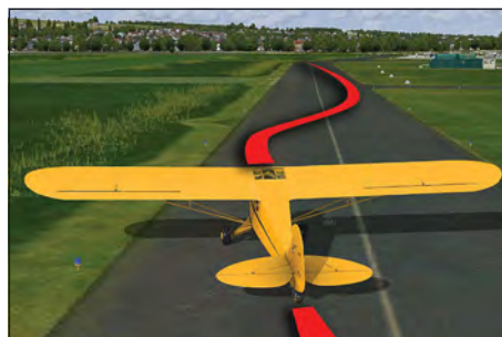
Fig 4 - With limited visibility over the nose, taildraggers usually taxi in a snaking pattern down the taxiways to check ahead
