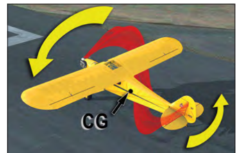
Fig 6 - The prop wash and rearward centre of gravity all conspire to make controlling a taildragger challenging
