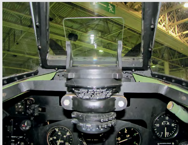
Above the instrument panel is an operable gunsight, with which you can dial in an aircraft's wingspan and distance. Again, compare this with the real thing below...
