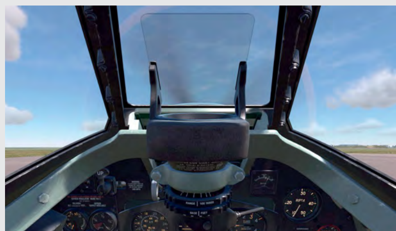
Above the instrument panel is an operable gunsight, with which you can dial in an aircraft's wingspan and distance. Again, compare this with the real thing below...
