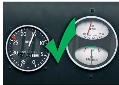
Before applying full power for take-off, check your oil temperature and pressure gauges to be sure all is well
