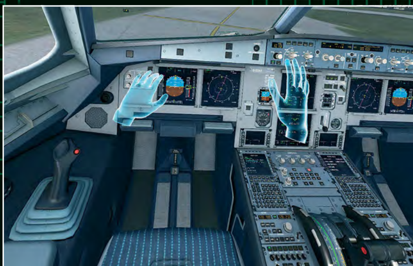
A Leap Motion sensor can be used to track the movement of your hands, enabling you to manipulate controls in the cockpit
