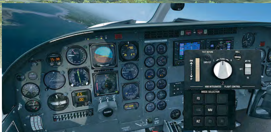
ABOVE LEFT: Though the panel has excellent readability, the 2D pop-up autopilot controller is a useful feature that allows for heads-up manipulation
