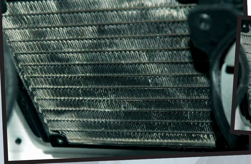
ABOVE: Dust in the radiator fins of a water cooler reduces its efficiency dramatically
