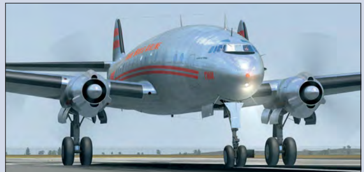
Connie sits high on its long undercarriage to ensure adequate ground clearance for the large propellers and to reduce the possibility of damage caused by debris
