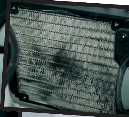
ABOVE: Dust in the radiator fins of a water cooler reduces its efficiency dramatically
