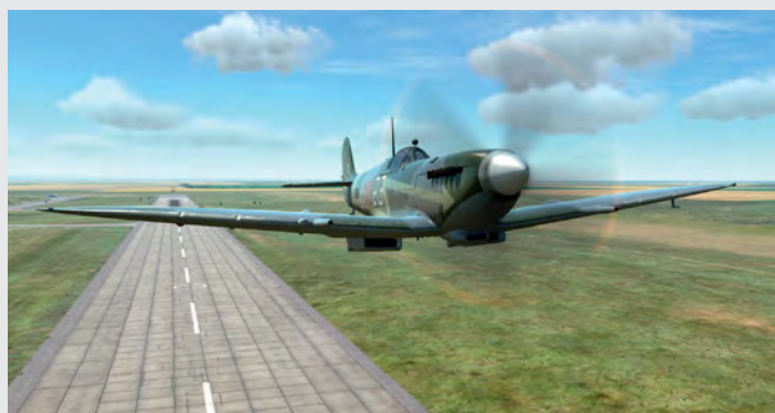
TOP: Take-off in the Spitfire presents a challenge and takes practice because of its narrow-track undercarriage and the torque created by the propeller pulling the aircraft to the left
